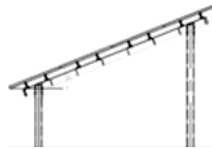
Double pole static structure with struts
