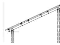
Double pole static structure with struts
